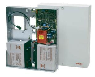
The NZ 300 LSN Intrusion Alarm Control Panel and the BE 300 LSN key pad ensure a high degree of flexibility and reliability. This is achieved through the use of the LSN Local SecurityNetwork. The Local SecurityNetwork LSN features a single, wire-saving transmission technology allowing all detectors and control elements of a security system to be connected to a danger detection system.
